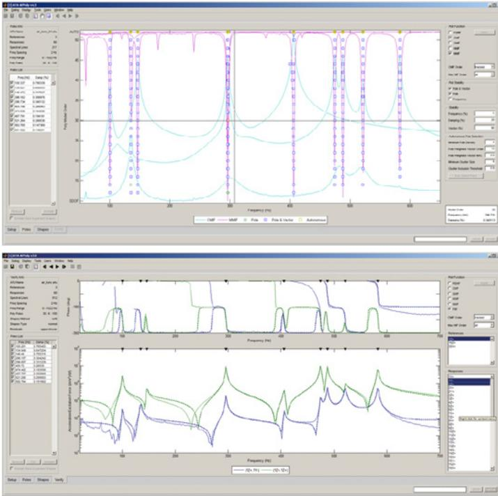
▲ Select poles from a stability diagram and overlay measured and synthesized FRF to verify the results.
