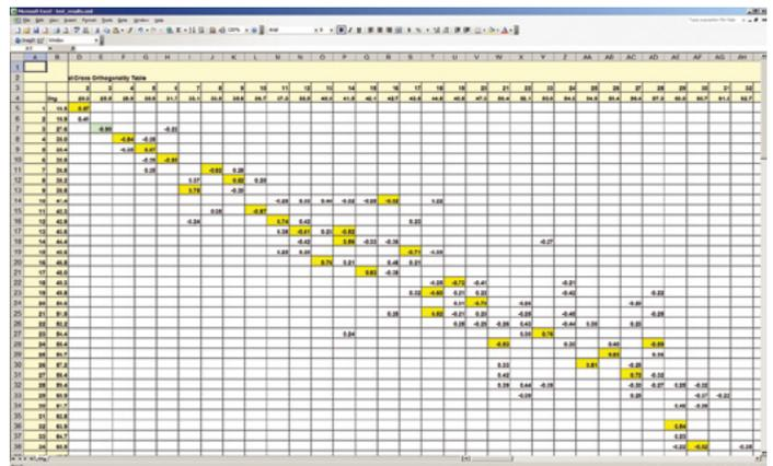
▲ MTK generates report-ready formatted test and analytical shape comparison output containing MAC and orthogonality comparisons.
