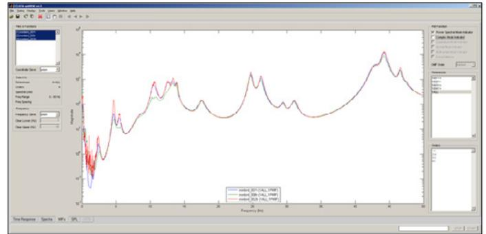
▲ Easily compare mode-indicator functions from multiple test runs.
