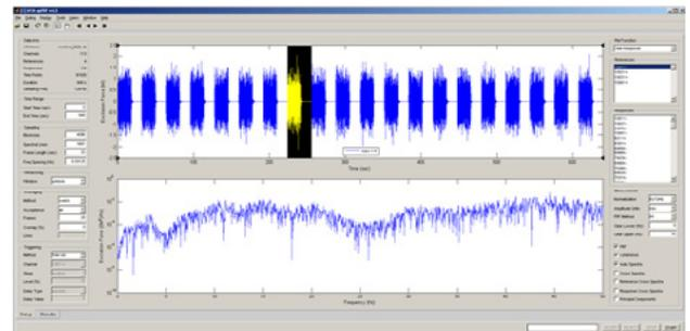
▲ Visualize and control processing of time-domain signals to the frequency domain with spFRF.
